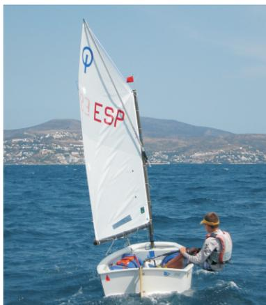
From 8 till 14 Knots you can pull the sheet until the boom is around 4-7 cm inside the hull corner in order to achieve more pointing angle (especially with the light and the medium models) . Please remember that you will have to ease the sheet when the boat is slowing down and trim it when the boat has speed.
